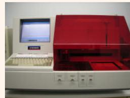
The plasma is placed into the Biochemistry Machine where it is mixed and incubated with various chemicals leading to colour changes which are converted to results by the machine.
